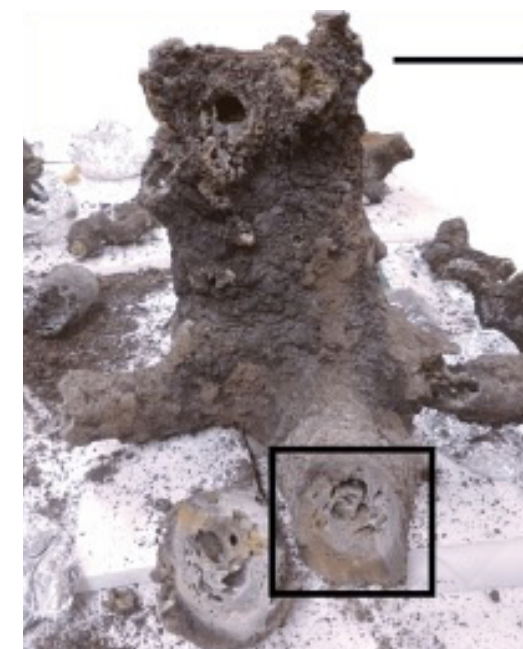
Main section of clay fulgurite created by lightning striking soil. Area of analysis indicated by box. Scale bar =10 cm
